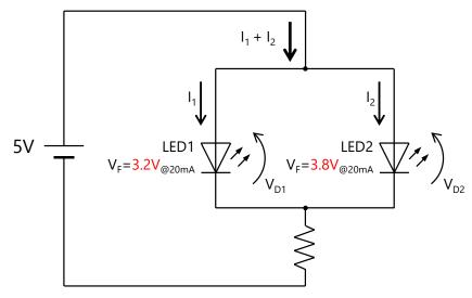
Figure 3. Circuit Diagram
