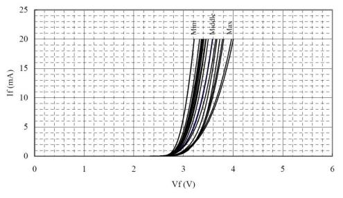
Figure 2. Forward Voltage - Forward Current
